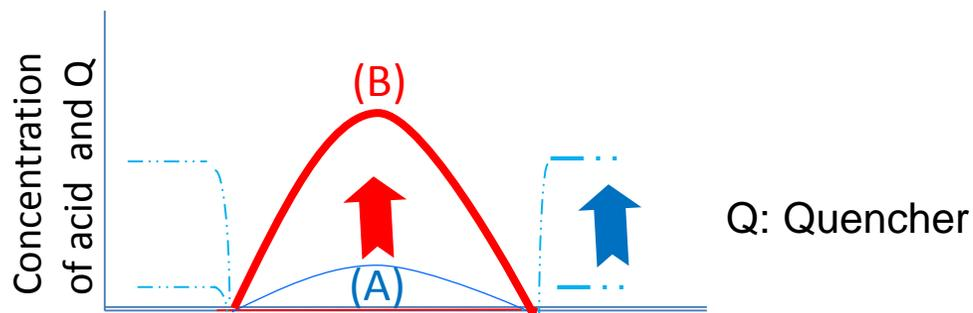
Schematic drawing of acid generation processes of PSCAR resist by the combination of 1<sup>st</sup> EB or EUV pattern exposure with 2<sup>nd</sup> photon flood exposure. The limitation of acid diffusion by high concentration quencher (Q) is necessary for high resolution pattern formation in PSCAR. Therefore, the **higher chemical gradient (dm/dx)** can be obtained.
