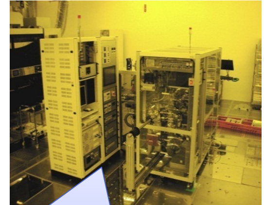
EUVOM-9000 (LTJ) E-gun based Qualification Tool
