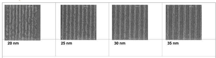
Sub 40nm lithographic features obtained under EUV exposure (at Sematech North) for the M21-based resist formulations. Dose: 48 mJ/cm<sup>2</sup>
