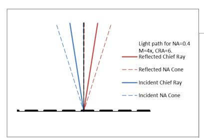
Current ML design can't support NA above ~0.33 at M=4.
