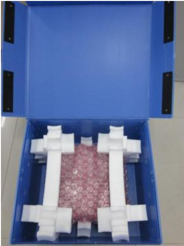
Inner box packed with pre-scanned reticle in Gudeng EUV-pod
