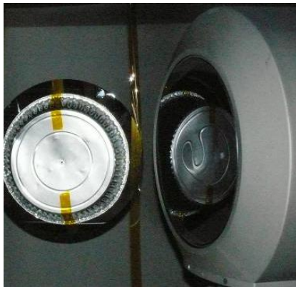
Pinhole camera installed in etch area
