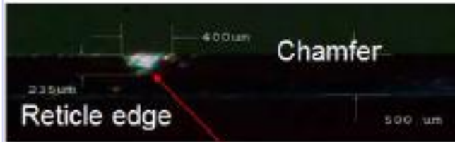
Damage in hold down pin area in reticle chamfer
