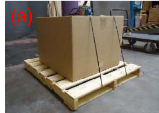
Palletized packaging for aPod, to reduce shipping shocks. It's about 12x bigger in volume than (b).
